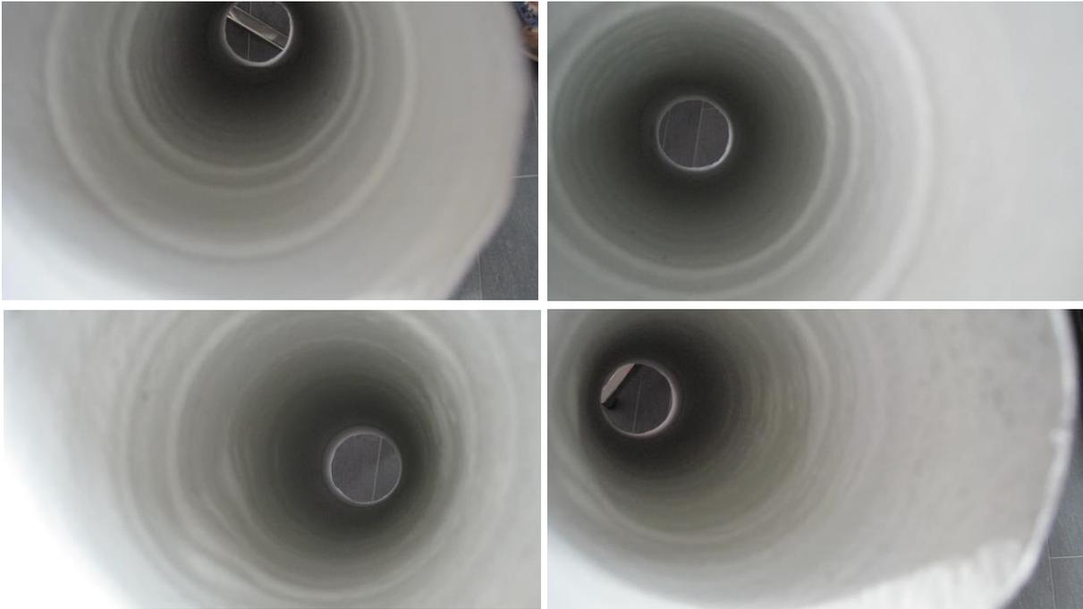
Photos Stainless steel flue gas discharge pipe (with rz-ecoseal) with a long term test that was carried out from 11-11-2017 to 21-3-2018, with 3158 operating hours of central heating.
